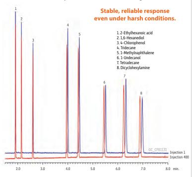
Column: Rxi"-5Sil MS, 30 m, 0.25 mm ID, 0.25 µm (cat.# 13623); Sample: Column test mix (cat.# 35226); Inj.: 1.0 µL split (split ratio 1:60), 4 mm recessed single taper (cat.# 20983); Inj. temp.: 250 °C; Carrier gas: helium, constant pressure; Linear velocity: 36 cm/sec @ 125 °C; Oven temp.: 125 °C; Det: FID @ 320 °C; Instrument: Agilent 6890
